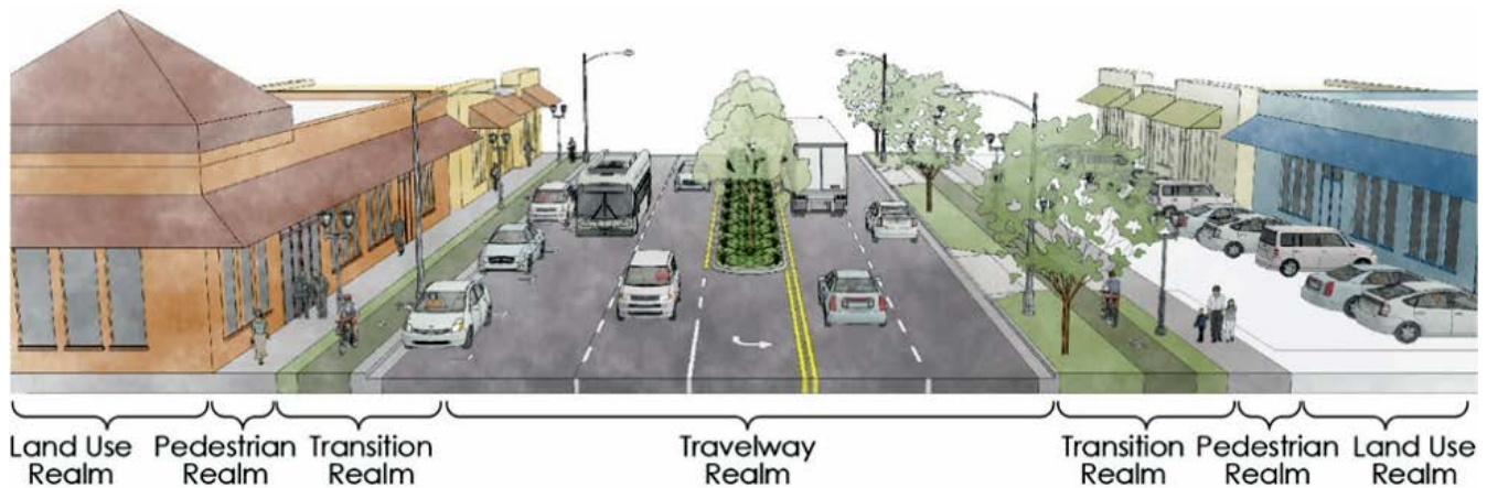
Figure 42. Illustration. Example of cross section realms.
